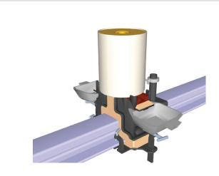
The arrangement for welding. The refractory sand mould is held in place around the rail with clamps. The disposable crucible is protected in a cardboard tube. Excess slag from the casting process flows into the slag pans.
