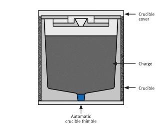
A section through the one-shot crucible. This is packed in a cardboard tube, which in turn is packed in sealed plastic film to prevent moisture ingress.
