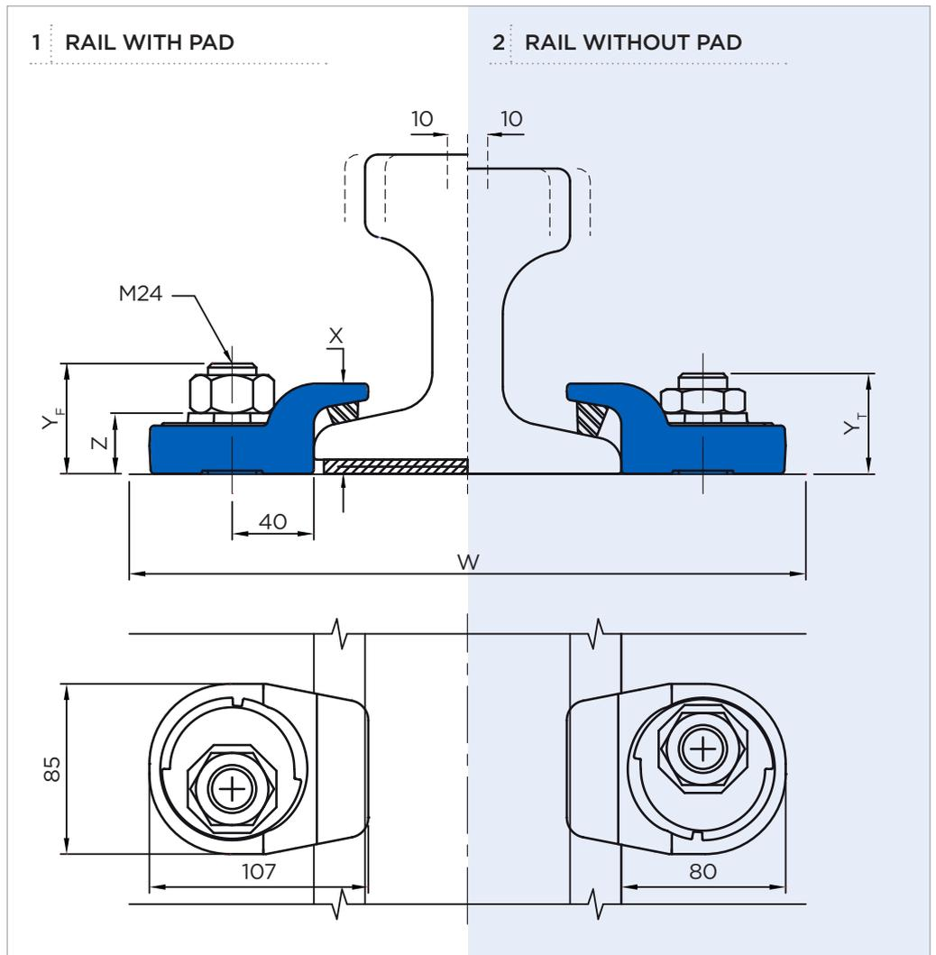
Minimum assembly width -  $W = \text{Rail width (F)} + 180\text{mm}$
