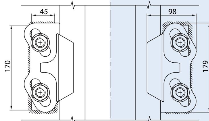
Minimum assembly width -  $W = \text{Rail width (F)} + 130\text{mm}$      $V = \text{Rail width (F)} + 22\text{mm}$
